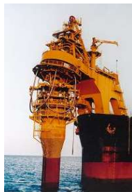
External Disconnectable Turret
