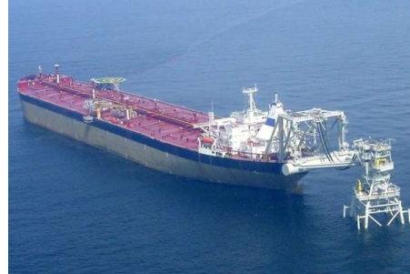
Kome Kribi FPSO w/ Tower Yoke Mooring System
