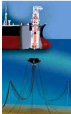
Internal turret with disconnectable buoy
