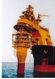
External Disconnectable Turret
